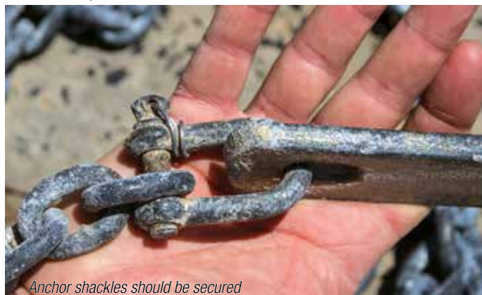
Anchor shackles should be secured
